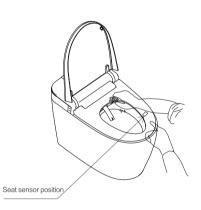
When checking all functions, make sure the seat sensor is covered and the energy saving icon or indicator light is off.
